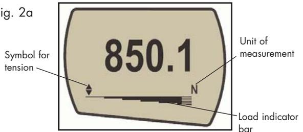
A load indicator bar alerts the operator to how much load has been applied to the transducer. As the load approaches the maximum rating of the transducer, the indicator bar changes appearance when above approximately 80% of the rated capacity. This warns the operator that steps should be taken to prevent excessive load being applied.
