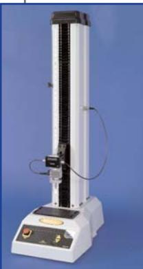
The MultiTest 5-*i* is a fully computer-controlled 5000 newton testing machine. Mecmesin Corporation's Emperor software enables users to develop sophisticated program routines and analyses to meet precise requirements for testing particular products. (Also available in a 1000 and 2500 newton capacity)
