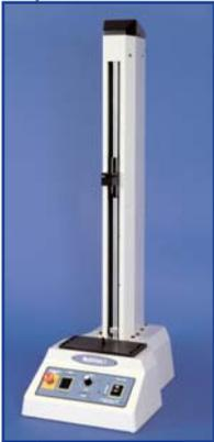
The MultiTest 1 is a budget-priced, potentiometer-controlled test stand with 1000 newton capacity. When used with a Mecmesin Corporation force gage and appropriate fixtures this system is ideal for relatively straightforward testing applications; the force gage captures maximum tensile and compressive loads. (Also available in a 2500 newton capacity)
