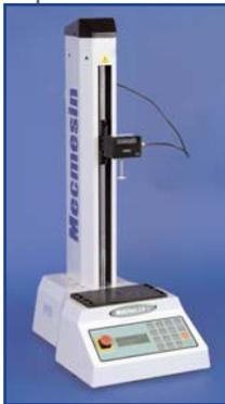
The MultiTest 2.5-*x* is a console-controlled 2500 newton stand, which can carry out simple test procedures and data analyses. Features include: cycling, load-holding, remote and running to a precise load, displacement, time or break. (Also available in a 1000 and 5000 newton capacity)
