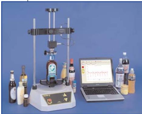
The Vortex-*i* is a fully computer-controlled motorized torque testing system. A Vortex improves reproducibility by allowing constant speed testing. However, a Vortex-*i* will enable complete control of the test procedure, analysis and reporting by using a new torque version of Mecmesin Corporation's powerful, flexible and user-friendly Emperor software.
